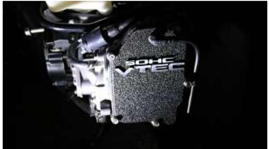
Place new Valve cover over cylinder head. Use 4 of the 5 supplied bolts to fasten valve cover. Place supplied 8 inch hose on Breather nipple on top of the valve cover. If hose is tight use dab of oil on barbed fitting so hose can slide on. Place last bolt through grommet and attach to valve cover. Feed hose through grommet facing down. Tighten
