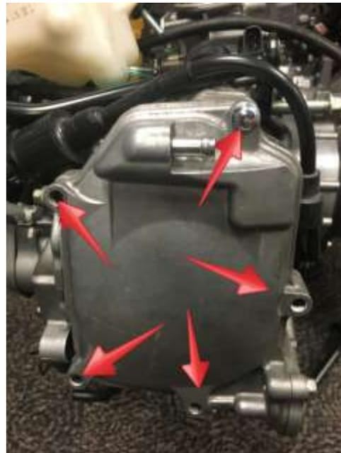
Once you remove the OEM Valve cover, flip it over and carefully remove the Valve Cover gasket and the O-ring as seen in above picture. You can use a toothpick, Paperclip, or any other object to remove gaskets, just be careful not to rip or cut them. Once removed. Place OEM gaskets in the NEW TRS Valve cover. If they are not sticking you may need to use a small amount of RTV to hold in place.
